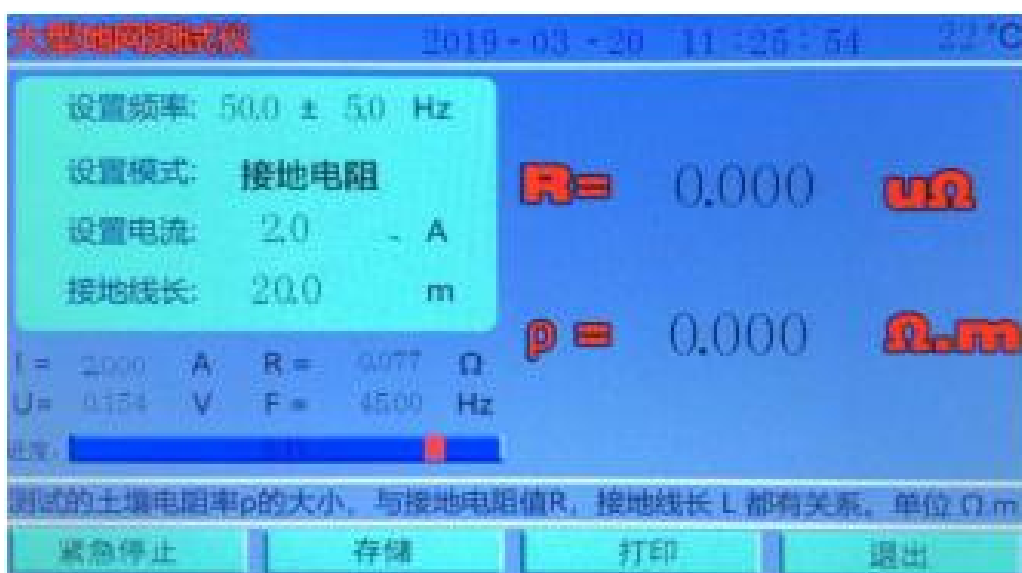
Figure 15 Ground resistance test interface
