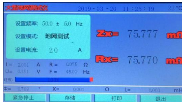
Figure 12 Ground network test result interface
